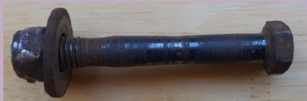
*Above: Worn rear suspension trailing arm bolt.*
